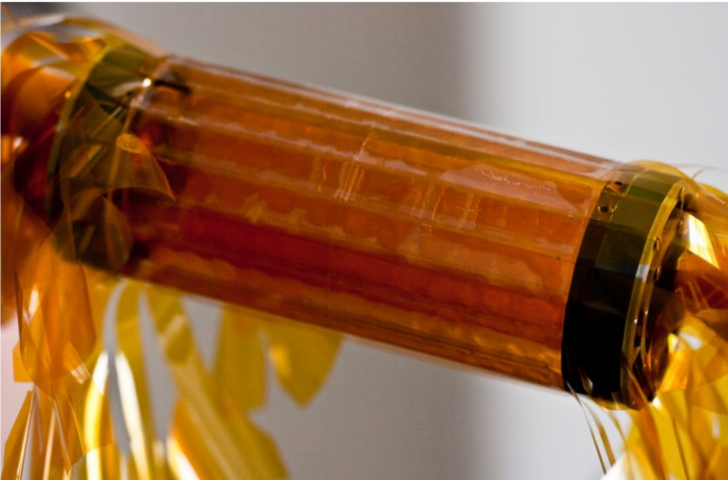
A 36cm long mock-up, equipped with 50 µm glass layers mimicking the pixels
